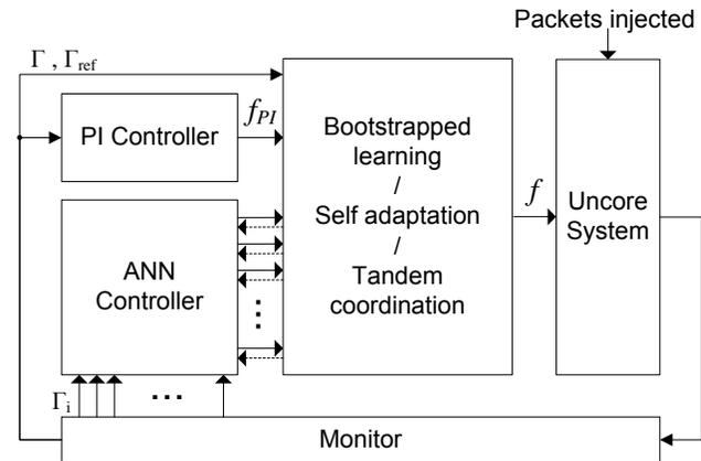
Figure 4: Architecture of the uncore DVFS control system.
