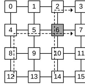
Figure 3: 16-core CMP in a  $4 \times 4$  2D mesh array. The darkened tile indicates location of the Power Control Unit (PCU). The dashed lines indicate paths traversing the NoC.
