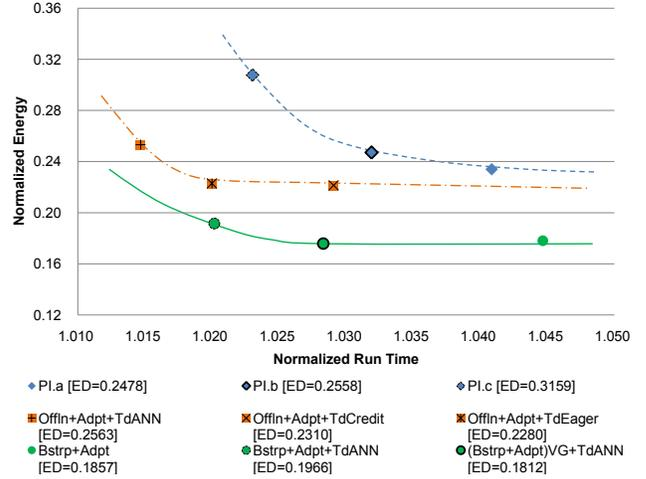
Figure 10: Pareto optimal points and normalized energy-normalized run-time curves for PI control-, offline-, and bootstrapped learning-based methods.
