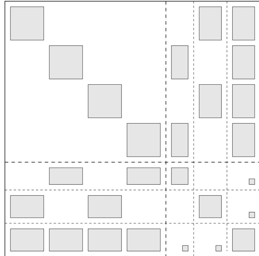
➤ For regular  $n \times n$  meshes, can show: fill-in is of order  $n^2 \log n$  and computational cost of factorization is  $O(n^3)$
