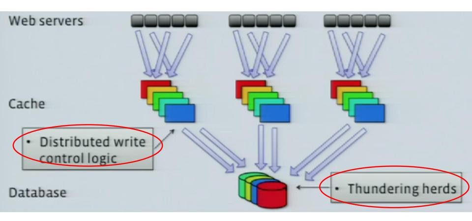
1. Complex distributed write logic to handle to ensure data correctness, consistency
