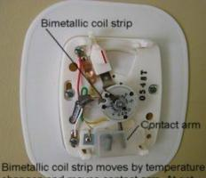
changes and moves contact arm. At set temp, arm moves to open or close contact
