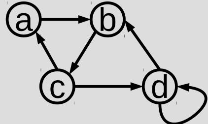
An adjacency matrix has a 1 in row i and column j if you can go from node i to node j
